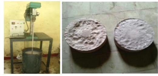
Figure 2. Machine and sample tests for concrete abrasion according to ASTM C1138 [27].
