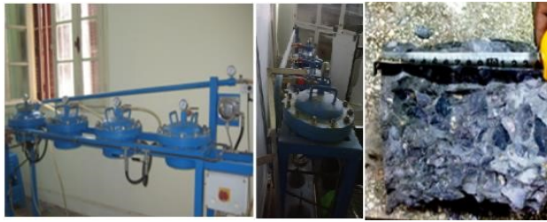
Figure 1. Sample of concrete after splitting tensile strength and measuring penetration.
