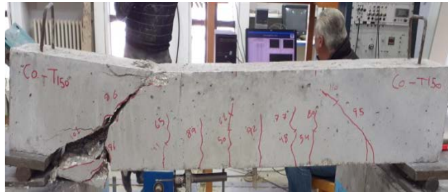
Figure 3. Typical failure mode of control beams.
