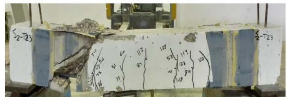
(a-2) 2 CFRP strips
