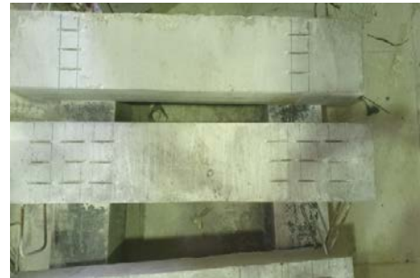
Drilling the grooves
