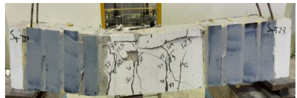
(a-4) 4 CFRP strips
