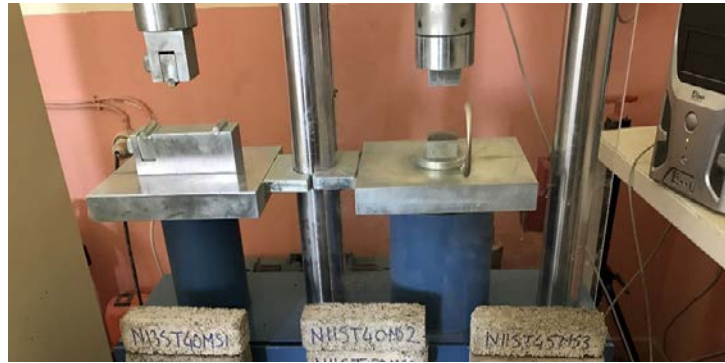
Figure 4. Compressive and flexural test device.
