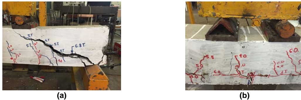
Figure 6. Failure modes of tested beams: (a) Diagonal tension failure, (b) Shear tension failure.
