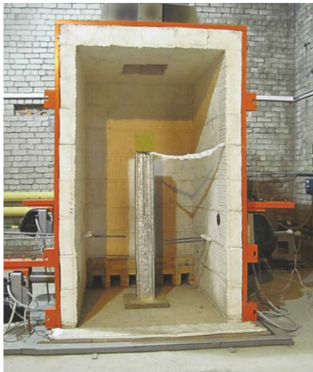
Figure 3. Fire Test Furnace
