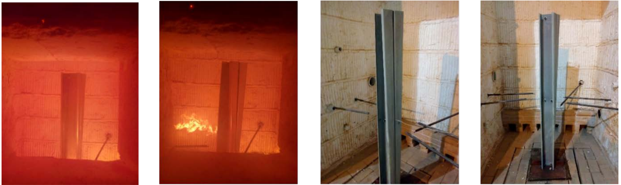
Figure 5. Unprotected prototype No. 1 during and after the test.
