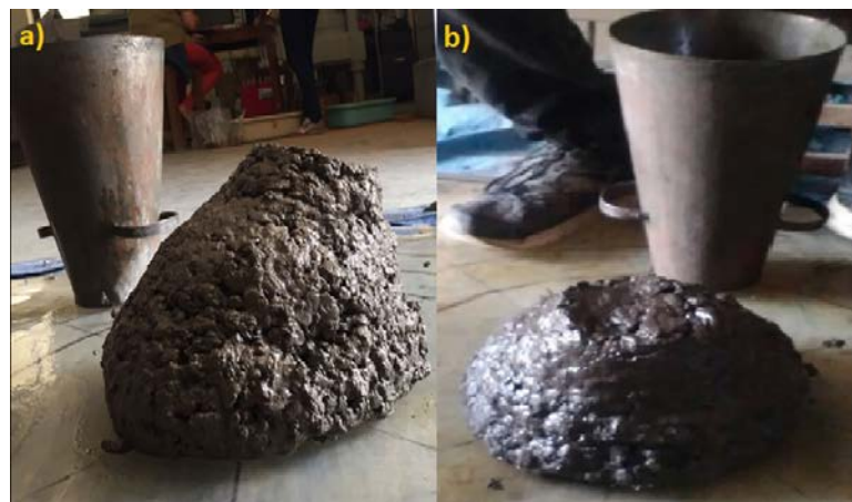
Figure 7. Slump in 100 % pond ash replacement a) without SP and b) with SP.
