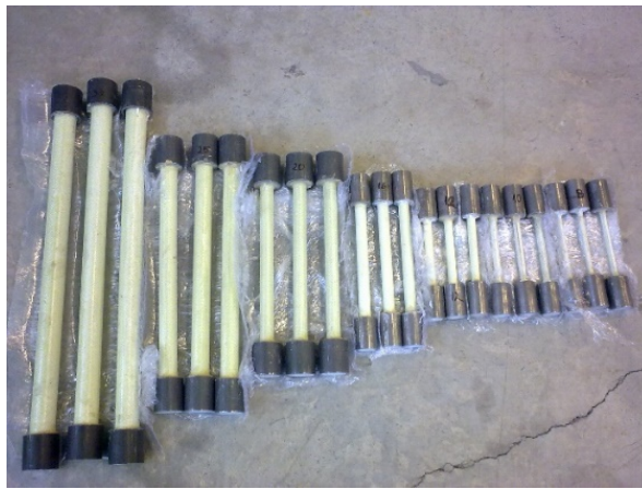
Figure 4. Bars for the compression test. Serie 2.
