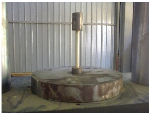
Figure 5. Compression test plate.
