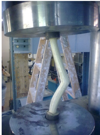
Figure 6. Compression test. Set of plates.
