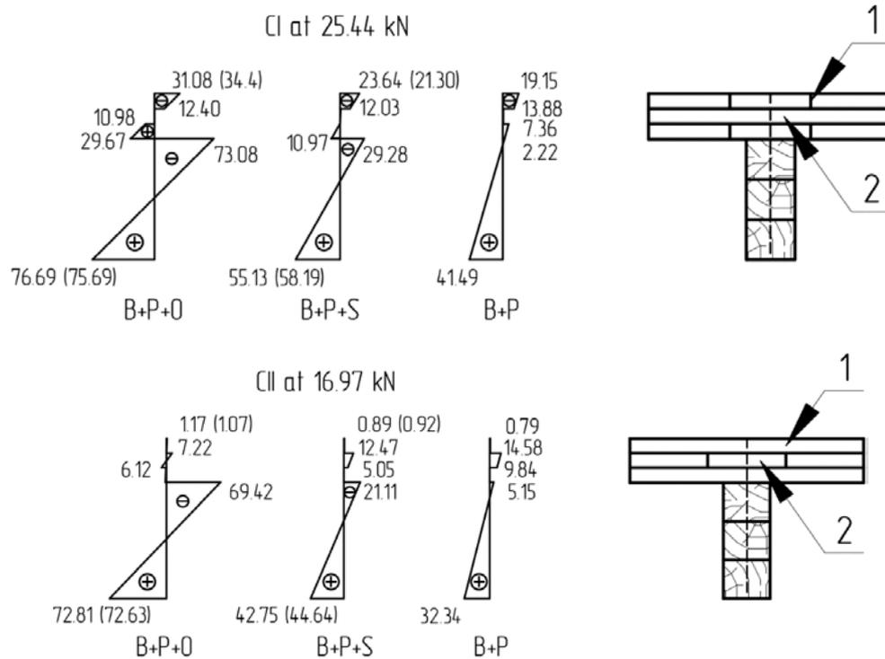
**Figure 5. Mid-span normal stresses distributions along cross-sectional depth of CI and CII composite structures: 1 – top layer of CLT panel; 2 – cross layer of CLT panel.**
