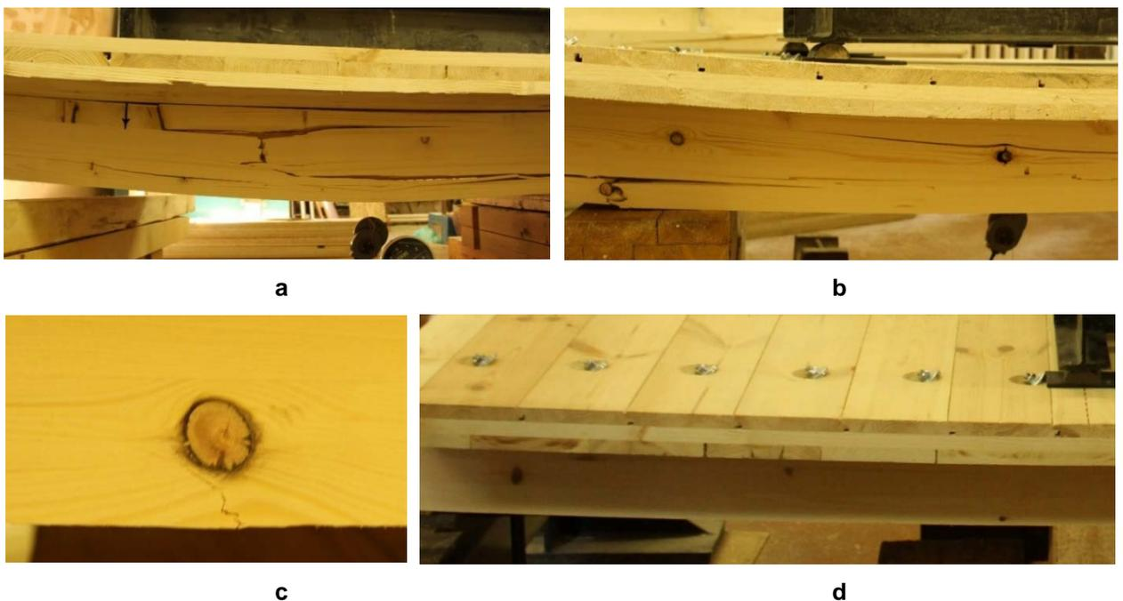
**Figure 6. Failure of the CLT-GLT composite structures: a – CI; b – CII; c – knot in the tensile zone of the GLT beam (CII); d – gap between lamellas of the CLT panel.**
