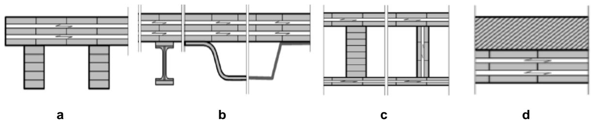
**Figure 1. Timber composite systems [1]: a – ribbed cross-section of the CLT-GLT structure; b – CLT with metal beams; c – box-shaped cross-section of the CLT-GLT structure; d – composite cross-section of CLT-concrete.**
