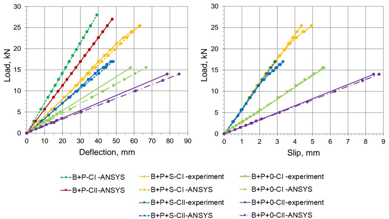
**Figure 4. Load-deflection and load-slip curves for the CLT-GLT composite structures bending tests.**
