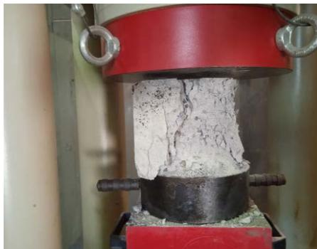
Figure 1. Testing a concrete cube at the hydraulic press ALPHA 3-3000S.
