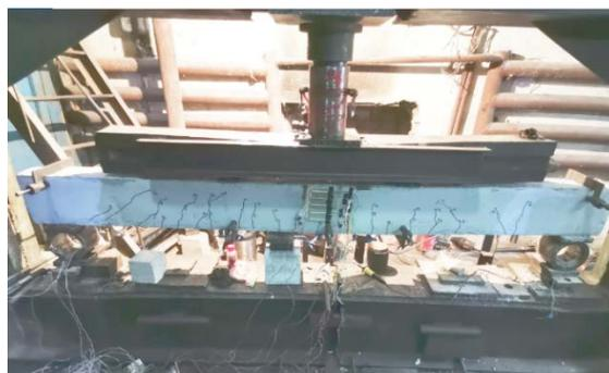
**Figure 4. General view of reinforced concrete beam tests.**
