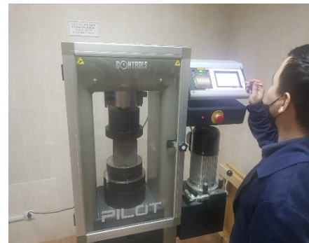
b) Compressive strength test
