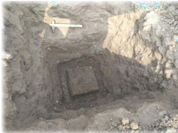
Figure 1. Collection of Undisturbed Soil Sample at 2-meter depth.
