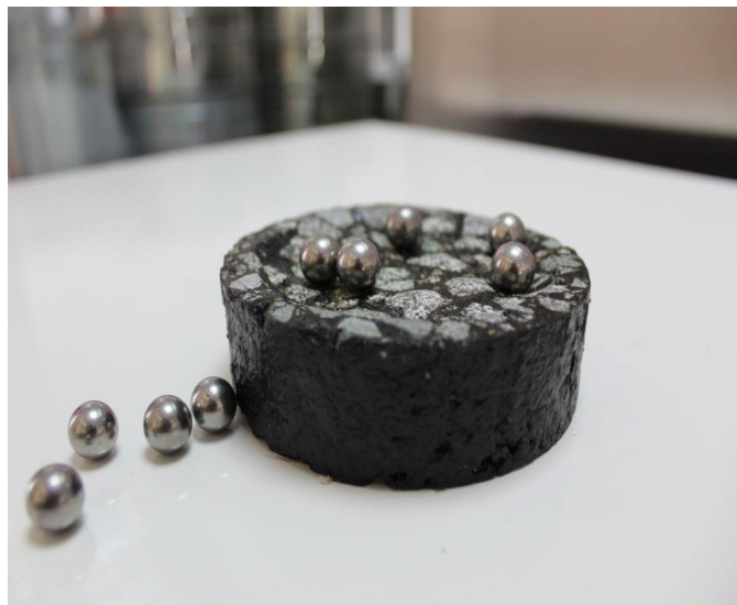
Figure 8. Asphalt sample with steel balls after testing.
