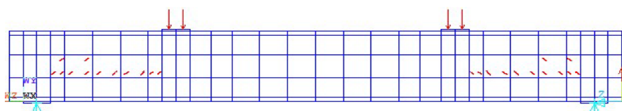
a) the beam starts to crack ( P_{crack}=22kN ), 3\phi 22
