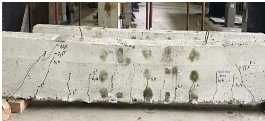
Figure 7. Formation and development of cracks in test beams.
