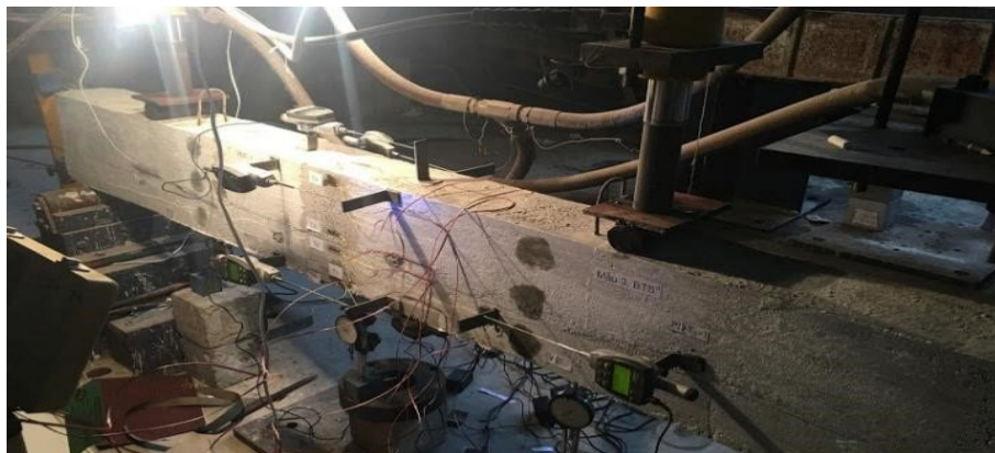
Figure 5. Test beams on the experimental pedestal.
