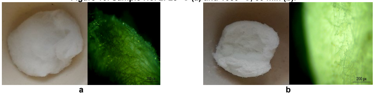
Figure 11. Sample No. 3: 25 °C (a) and 1050 °C, 30 min (b).
