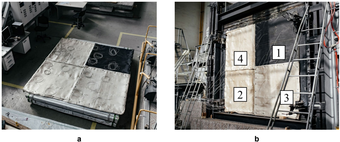
Figure 4. Installation of the combined sheet in the furnace opening: (a) appearance of the sheet before testing with attached thermocouples (b) side view.
