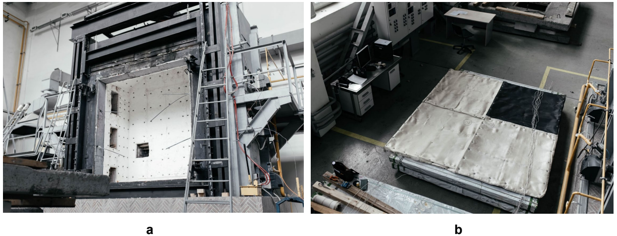
Figure 3. Preparation for the test: a) furnace; b) assembly of the combined web on the stand.
