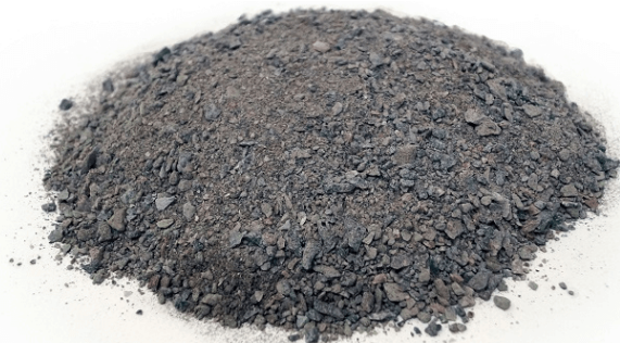
Figure 3. Appearance of granite crushing screening.
