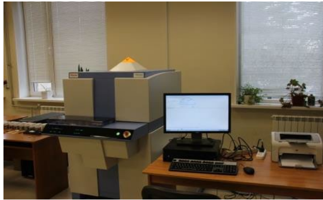
Figure 7. Spectrometer "ARL 9900 WorkStation".
