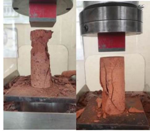
Figure 18. General view of cylindrical samples at failure after UCT, compiled by the authors.
