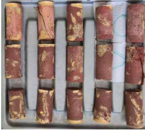
Figure 17. General view of cylindrical samples at failure after TXT, compiled by the authors.
