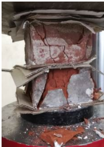
Figure 15. General view of the brick samples at failure, compiled by the authors.
