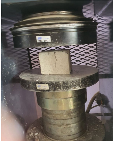
Figure 2. AAC cube for compressive strength test.
