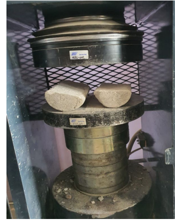
Figure 3. AAC cylinder for tensile strength test.
