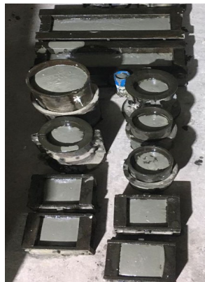
(a) Samples after casting
