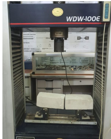
Figure 4. AAC prism for flexural strength test.
