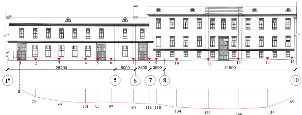
Figure 13. Diagram of the accumulated settlements across wall A. The values are given in millimeters 5 .
