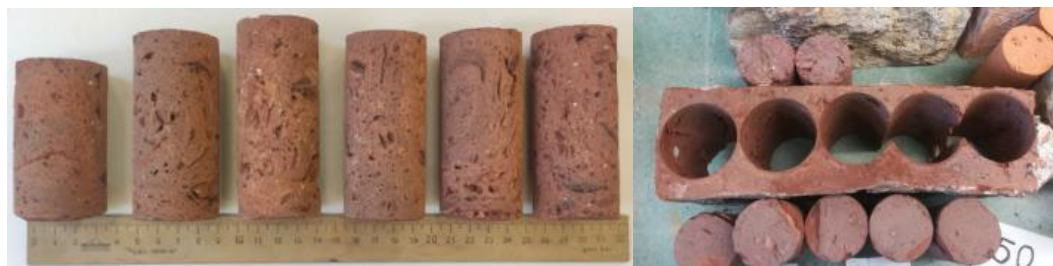
Figure 10. Cylindrical samples prepared for TXT and UCT, compiled by the authors.
