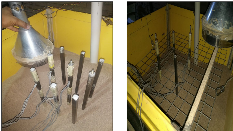
Figure 5. Raining tool and positions of the piles within steel mesh.
