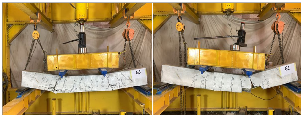
Figure 6. Crack pattern of the beams G1 and G3.
