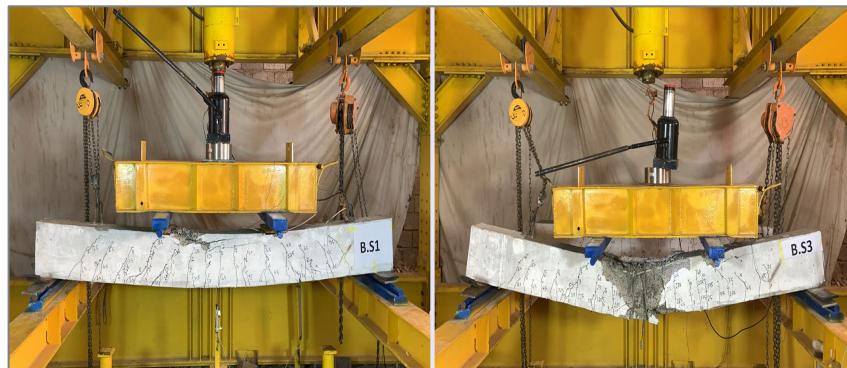
Figure 4. Crack pattern of the beams B.S1 and B.S3.
