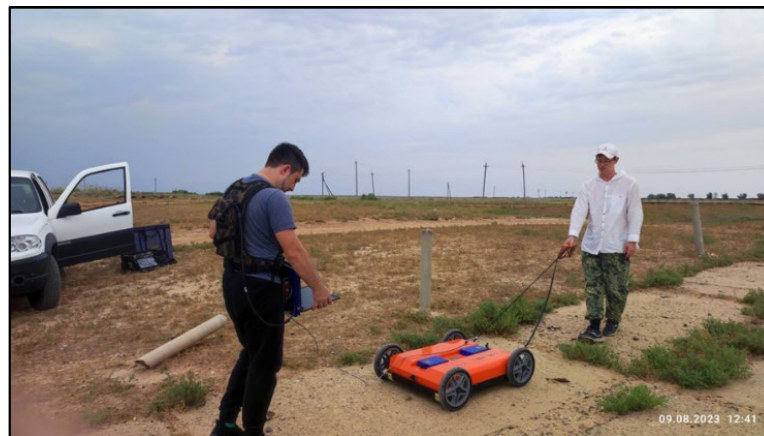
Figure 5. The GPR survey.
