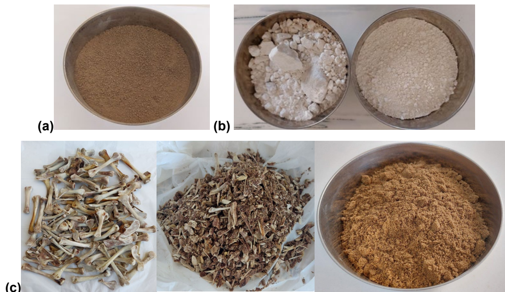
Figure 1. The materials used (a) clayey soil, (b) limestone, and (c) waste chicken bone.
