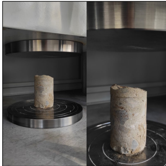
Figure 4. Testing of a core sample using a universal testing machine MIM.4-1000.
