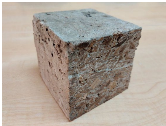
Figure 2. Appearance of the finished sample of group 4 for research (the side surface is cut off at the front to visualize the interior distribution of crushed TMW filler).
