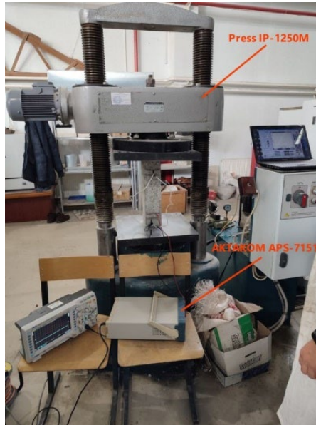
Figure 2. Photo of mechanical testing and electrical resistivity measurements.
