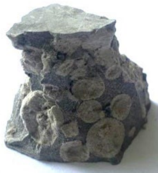
Figure 6. Mortar sample chipping with granular aggregate 2.5 mm fractions.
