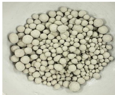
Figure 4. Granulated aggregate, obtained in a laboratory facility.
