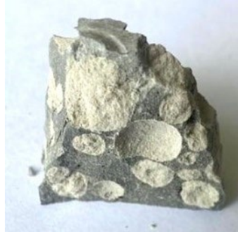
Figure 8. Mortar sample chipping with granular aggregate 10 mm fractions.
