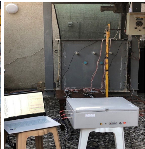
e) data logger and computer to save test data
