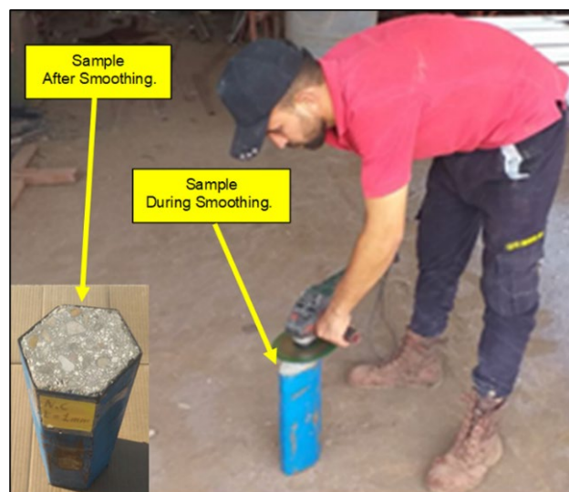
Figure 13. Shows smoothing surfaces of some samples.
