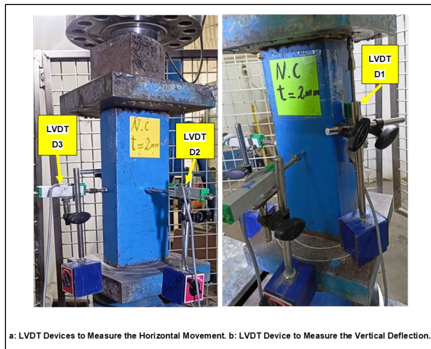
Figure 14. Location of LVDT devices on RACFST column with a rectangular cross-section under the test.
