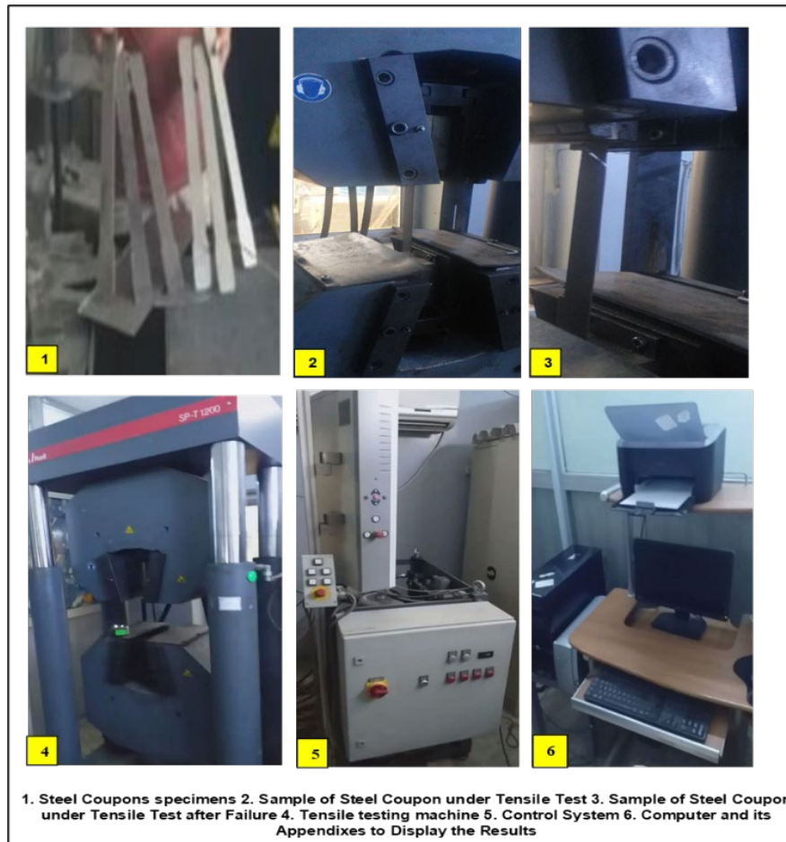
Figure 8. Setup of steel coupons for a typical tensile test and types of equipment, and devices used.
