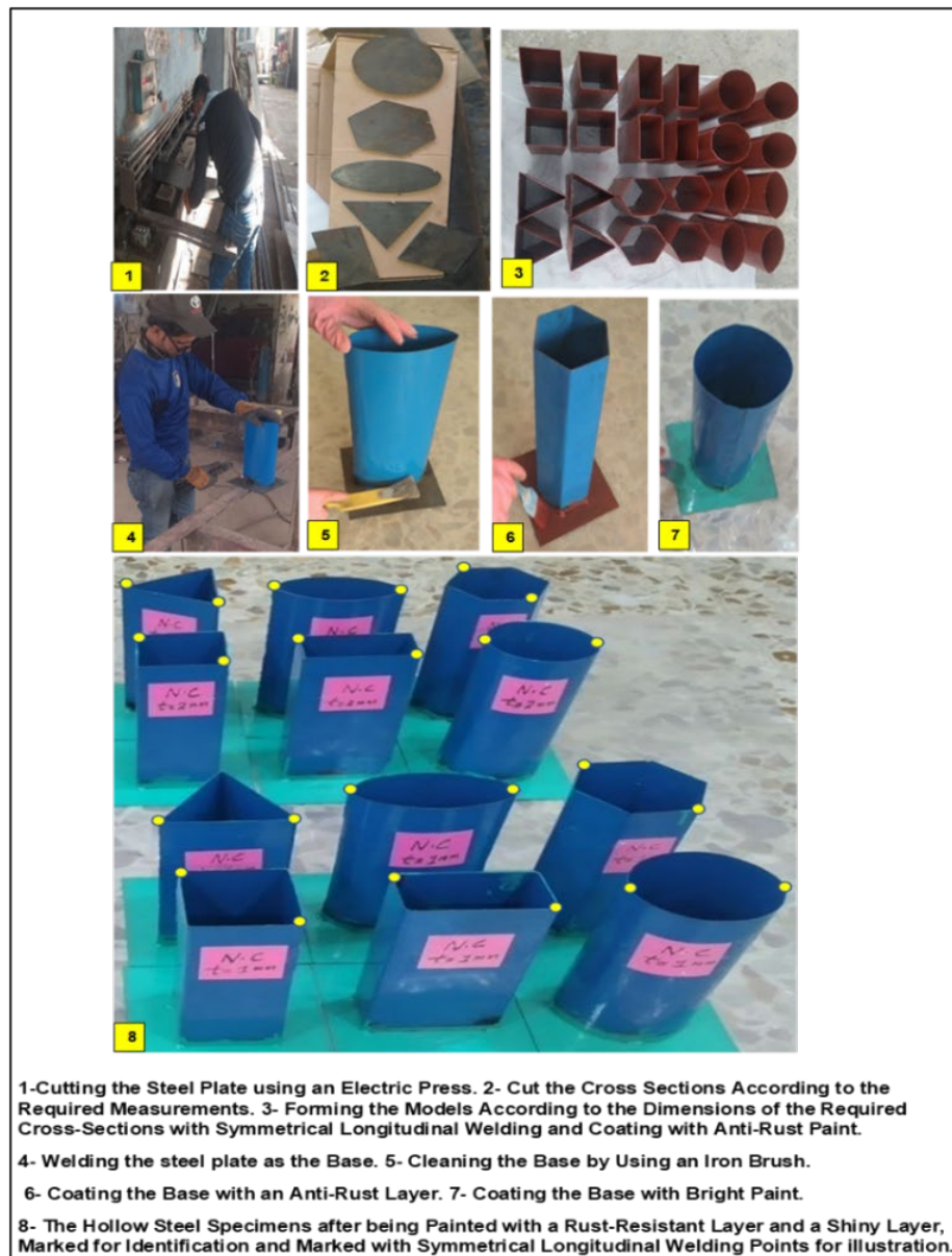
Figure 10. Manufacturing steps of hollow steel tubes and types of equipment used.
