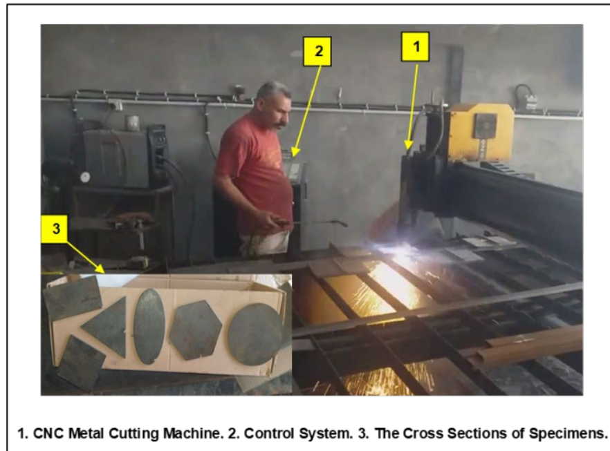
Figure 9. Shows the CNC metal cutting machine setup, control system, and devices used, with cross-sections of specimens and other parts.
