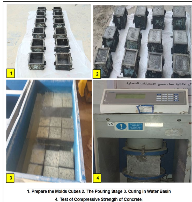
Figure 5. Steps of three mixing trials of concrete to achieve the target compressive strength.
