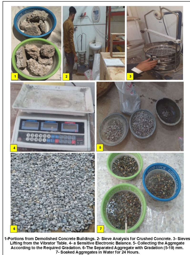
Figure 4. Preparation stages of recycled coarse aggregate and devices used.
