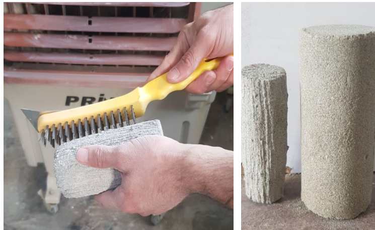
Figure 3. Photographs of the durability test specimens.
