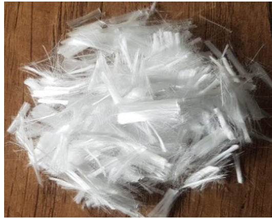
Figure 2. Photograph of polypropylene discrete fiber (12 mm).
