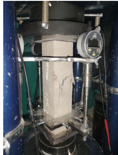
Figure 2. The state of the sample after the first (left) and last (right) loading cycle at a temperature of 600 °C.
