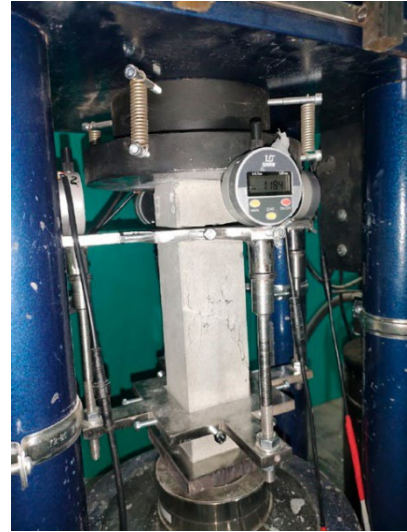
Figure 1. The state of the sample after the first (left) and last (right) loading cycle at a temperature of 20 °C.
