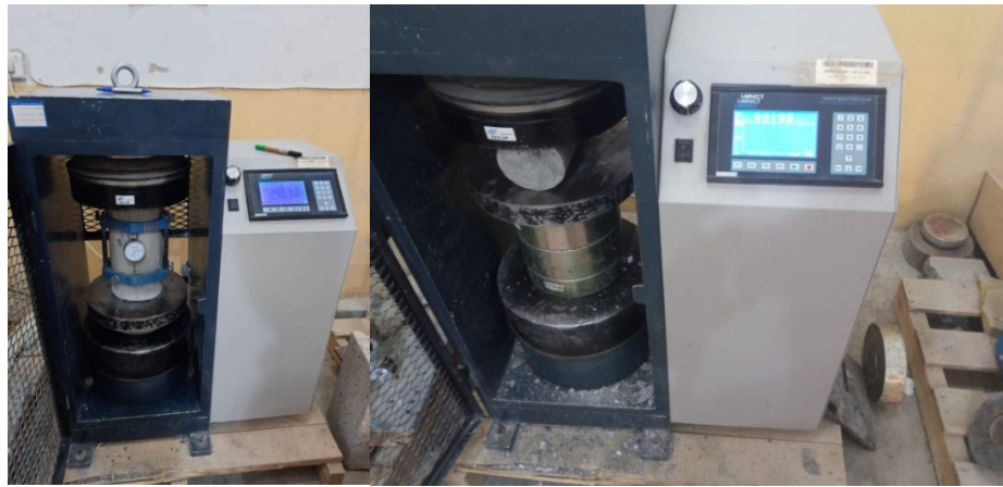
Figure 6. Specimens under modulus of elasticity and tensile strength tests.
