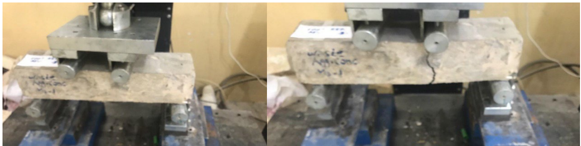
Figure 4. Flexural strength test shows ductile failure for white ceramic aggregate concrete.
