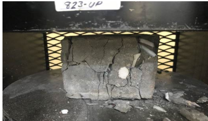
Figure 3. White waste ceramic concrete after compression test.
