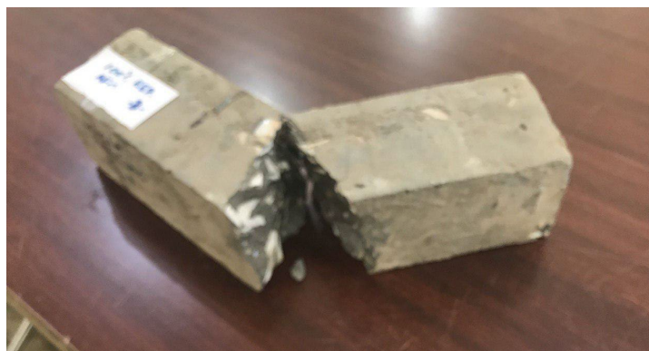
Figure 5. 100 % white ceramic as waste aggregate (replacement) after flexure test.
