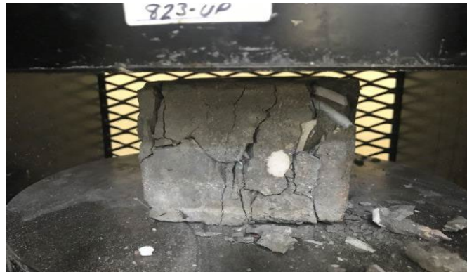
Figure 3. White waste ceramic concrete after compression test.
