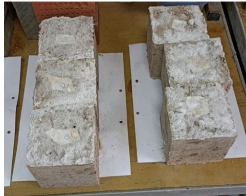
Figure 2. 100×100×100 mm cube samples with fluoroanhydrite to loam ratio 40:60 by weight.
