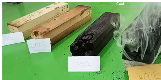
Figure 5. Specimens after exposition to different heating rates, during 60 min.
