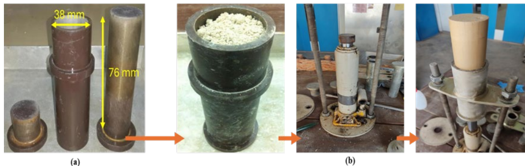
Figure 3. Procedure of kaolin preparation.
