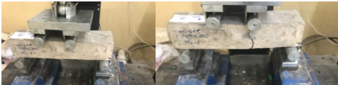
Figure 4. Flexural strength test shows ductile failure for white ceramic aggregate concrete.
