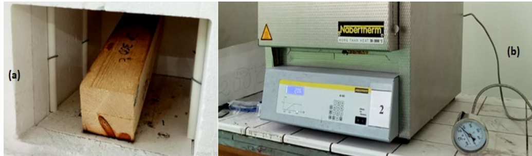
Figure 2. Type of furnace used: (a) specimen in 300 °C heating, (b) furnace containing a sample with a thermocouple.
