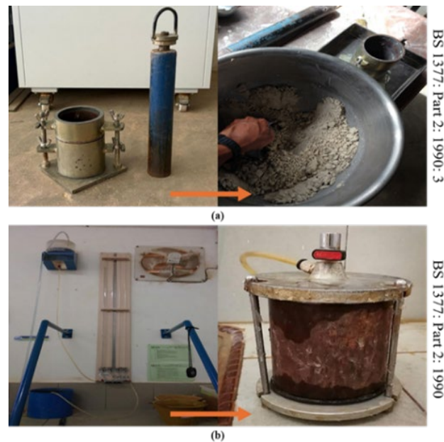
Figure 5. Mechanical experiments (a) Standard compaction (b) falling head test.
