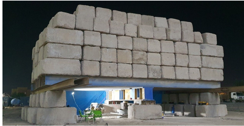
Figure 6. Static load test in-situ.
