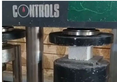
Figure 6. Compressive strength test.
