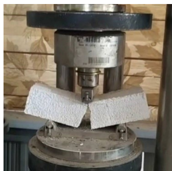
Figure 7. Flexural strength test.
