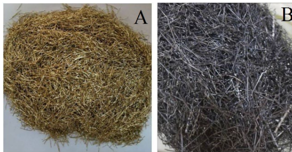
Figure 2. Types of steel fiber: (A) straight and (B) with hooked ends.
