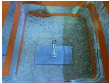
a. Compaction of soil at 5 cm layer
