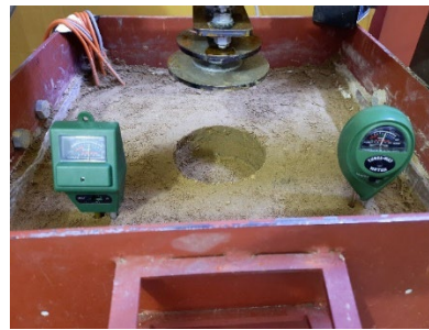
f. Preparing a model at depth foundation ( D_f = 0.5 B or 1.0 B )
