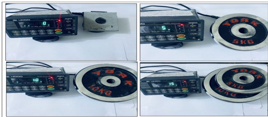
Figure 4. Load Cell Calibration steps.
